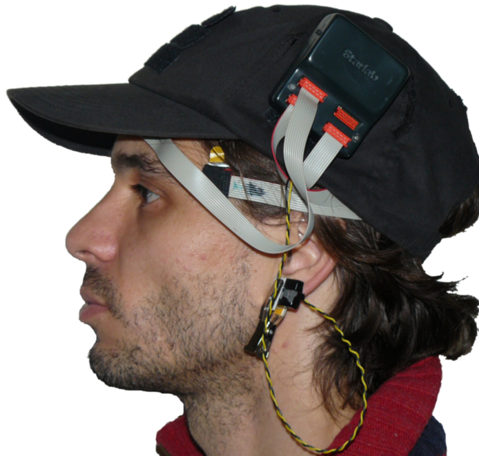
Fig. 1.1 ENOBIO 4 lead sensor integrated in a cap. In this picture only 3 channels are connected (grey cables). We can also see the common mode cable connected to the left ear lobe of the subject (black and yellow cable). The ENOBIO sensor is valid for recording EEG and ECG, but it can also measure electrooculogram (EOG) and electromiogram (EMG).
